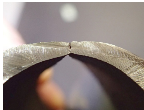
Fig. 7. TO2, changing thickness of pipe
